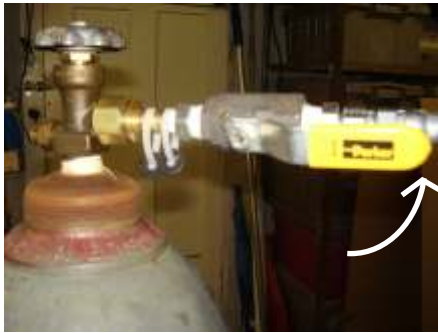
Ball valve shown in ON position
