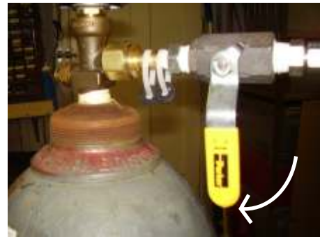
Use 11/8" wrench to tighten fitting to tank. Note ball valve shown in OFF position
